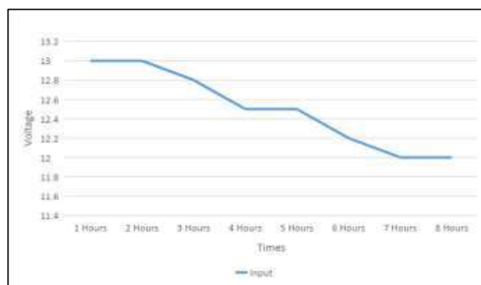
Figure 7: Input Voltage of Inverter depends on hours usage
